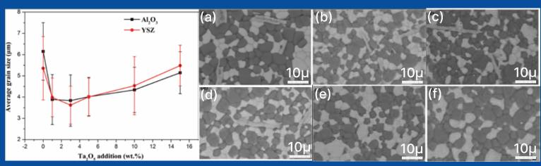
Figure 5: Resultant Ta<sub>2</sub>O<sub>5</sub> Addition Effect on YSZ and Al<sub>2</sub>O<sub>3</sub> Average Grain Size (left) and Corresponding YSZ Micrographs from Low (a) to High (f) Ta<sub>2</sub>O<sub>5</sub> Addition (right) Among 0, 1, 3, 5, 10, and 15wt% Ta<sub>2</sub>O<sub>5</sub> Dopant Concentrations
