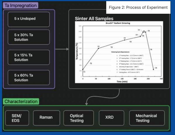
Figure 2 Outlines Investigatation of [Ta] Influence on Mechanical, Optical, Phase, and Morphological Properties. Ta-YSZ synthesis is Irrelevant to this Experiment
