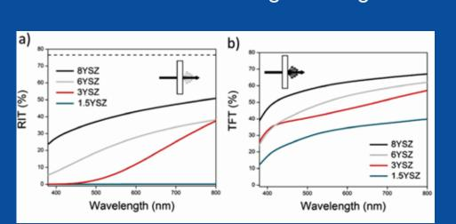
Figure 11: Real In Line (RIT) and Total Forward Transmission (TFT) of 1.5mol% - 8mol% Yttria Concentrations in YSZ, Revealing Translucency
