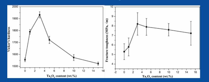
Figure 6: Effect on Vicker's Hardness (left) and Fracture Toughness (right) Among 0, 1, 3, 5, 10, and 15 wt% Ta<sub>2</sub>O<sub>5</sub> Dopant Concentrations.
