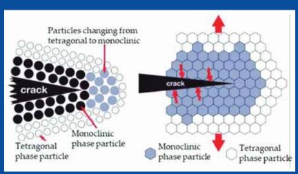
Figure 12: M Phase Transformation Toughening
