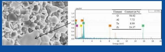
Figure 4: Quantitative Spectra EDS Suggesting Spatially Ta-Zr-O Distinct Phase Precipitation Among Ta<sub>2</sub>O<sub>5</sub> Doping
