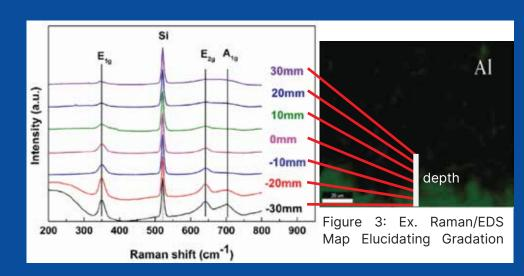
and determine penetration depth and gradation profile in Ta-Doped cross-section through corroborated Peak Transformation Analysis
