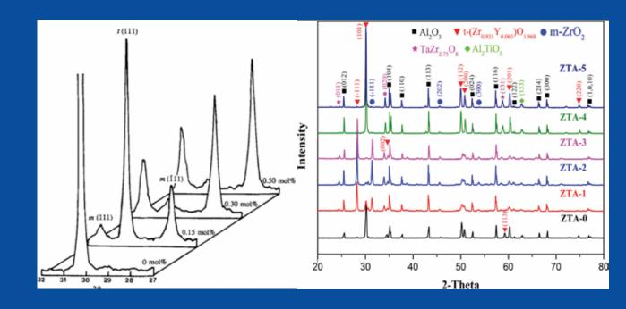
Figure 7: Increasing Ta<sub>2</sub>O<sub>5</sub> concentration's inverse effect on tetragonal YSZ phase stability (left), and significant TaZr<sub>2.75</sub>O<sub>8</sub> phase precipitation (right) for YSZ toughened alumina (ZTA) of increasing (ZTA-0 to 5) Ta
