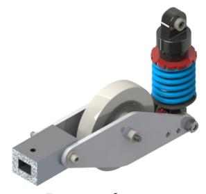
**Dynamics** The stabilization system is composed of 8 components. These components work in tandem to provide a lateral and vertical settling time of 0.47 seconds in response to a 1 cm disturbance.
